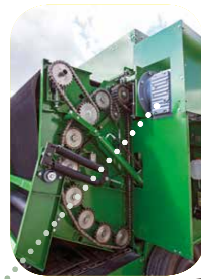
Direct drive of the baler chamber
