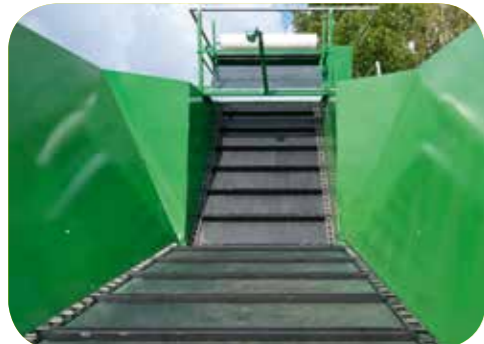
Feed hopper with elevator chain
